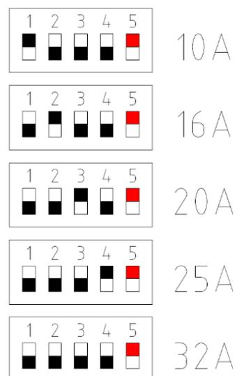
Microswitch 5 must always be switched on, as this will switch on the DC 6mA sensor and the circuit breaking function!
